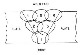
Figure 3-15.—Weld layer sequence.
