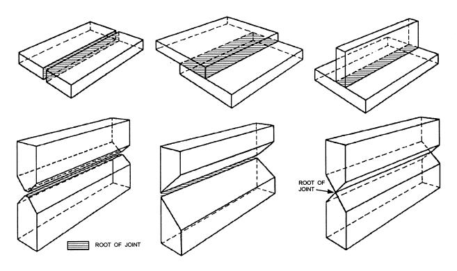
Figure 3-7.—Root of joint.
