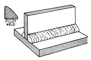
Figure 3-26.—T ee joints.
