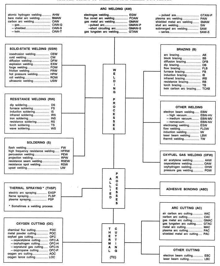
Figure 3-1.—Welding processes.
