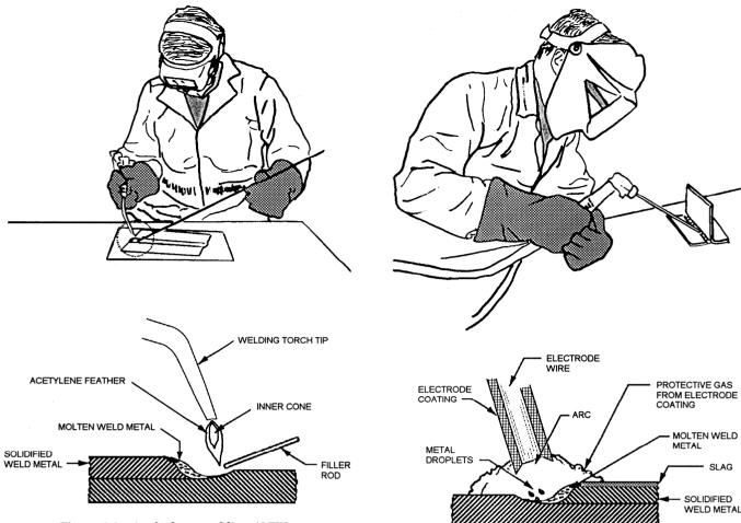
Figure 3-2.—0xyfuel gas welding (OFW).
