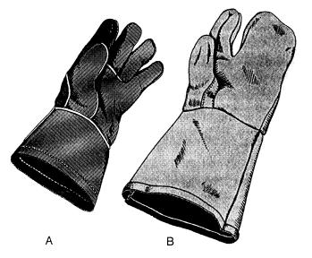
Figure 3-57.—Welding gloves and mitts.
