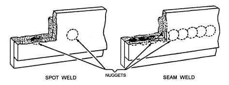
Figure 3-19.—Spot and seam welds.
