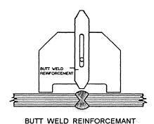
Figure 3-21.—Using a welding micrometer.
