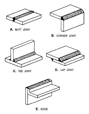
Figure 3-6.—Basic weld joints.
