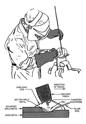
Figure 3-4.—Gas tungsten arc welding (GTAW).
