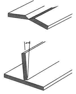
Figure 3-36.—Allowing for distortion.
