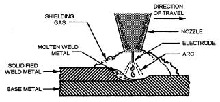
Figure 3-5.—Gas metal arc welding (GMAW).
