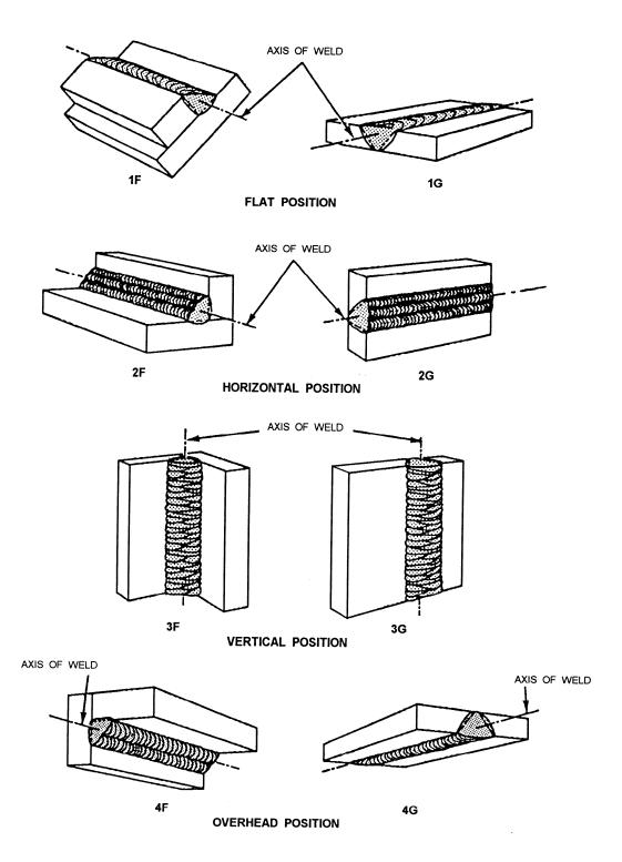
Figure 3-29.—Welding positions—plate.
