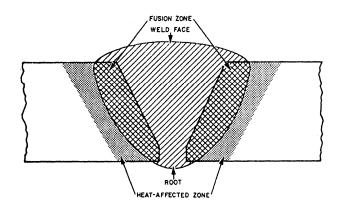
Figure 3-22.—Zones in a weld.
