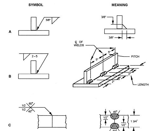
Figure 3-50.—Dimensioning of welds.
