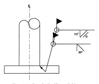
Figure 3-55.—Example of welding symbol in use.
