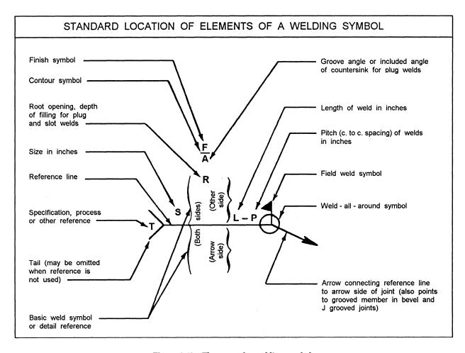
Figure 3-48.—Elements of a welding symbol.
