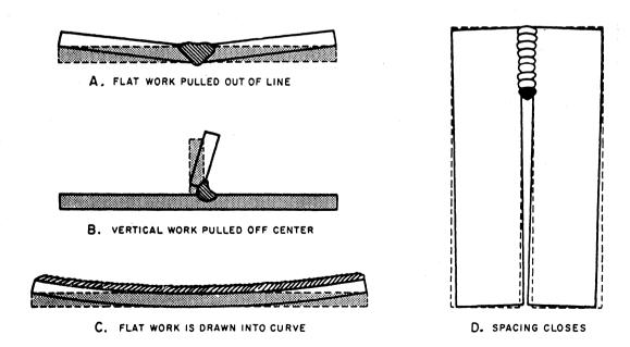
Figure 3-32.—Distortion caused by welding.
