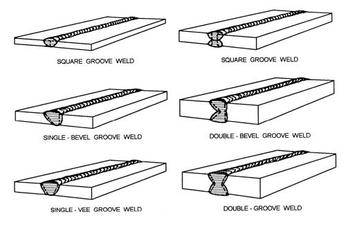
Figure 3-13.—Standard groove welds.
