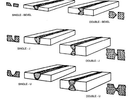
Figure 3-24.—Additional types of groove welds.
