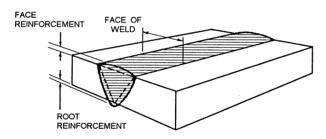
Figure 3-11.—Weld reinforcement.
