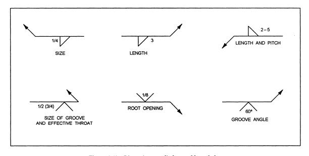
Figure 3-49.—Dimensions applied to weld symbols.
