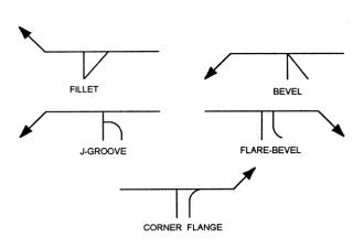
Figure 3-45.—Weld symbols applied to reference line.
