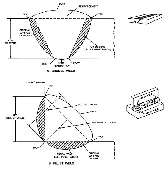
Figure 3-20.—Parts of a groove weld and fillet weld.
