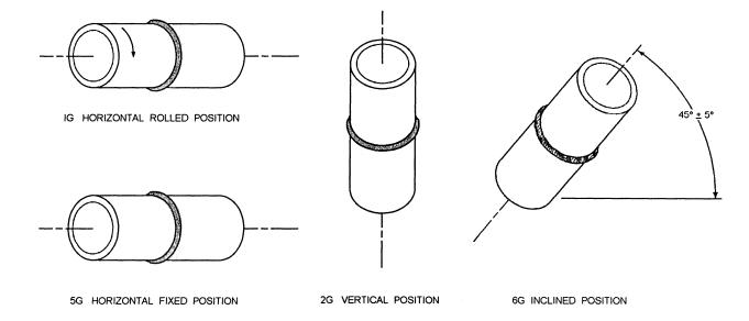
Figure 3-30.—Welding position-pipe.
