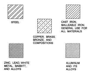
Figure 3-39.—Section lines for various metals.
