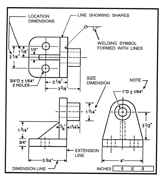
Figure 3-40.—Elements of an orthographic drawing.
