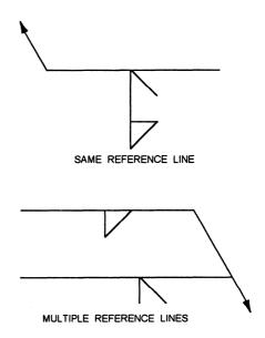
Figure 3-54.—Representing multiple welds.
