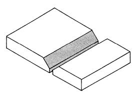
Figure 3-23.—Butt joints.
