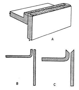
Figure 3-28.—Flanged edge Joints.
